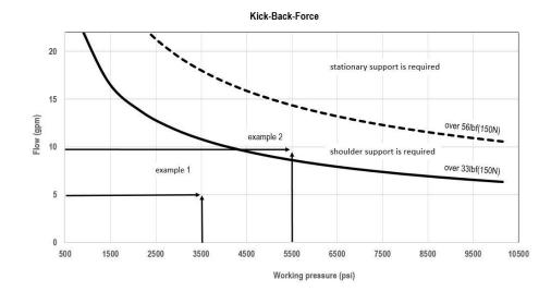
Example 1: For a flow rate of 4 gpm ( 15 l/min ) and an operating pressure of 2900 psi ( 200 bar ), the recoil force is less than 33lbf ( 150 N ). No further measures are needed.
